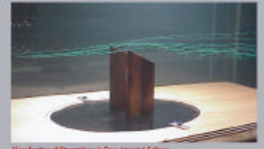
Visualization of Streamlines in Flow, Imperial College
