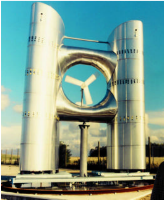
Figure 9: Photograph of the Prototype UWECS Building (Wind Concentrator) during Field-Testing
